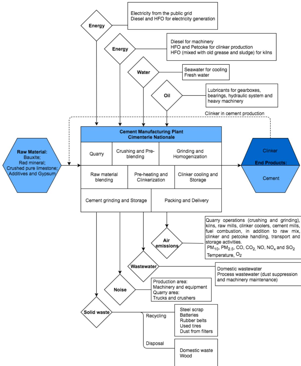
Figure 1. CN mass flow diagram
